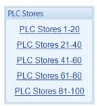
The selected section displays the value currently set for each *Store* an provides the user with the ability to change that value. *Stores* are used within the module's PLC to affect mathematical equations or change set points within the created PLC functions.
