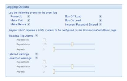
NOTE: Sending events by SMS is only available when the module is configured to communicate to a supported modem by RS232. Refer to section entitled *RS232 Port* elsewhere in this document for further details.
