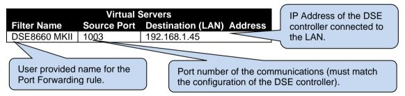
**Result :** Traffic arriving from the WAN (internet) on port 1003 is automatically sent to IP address 192.168.1.45 on the LAN (DSE module) for handling.
