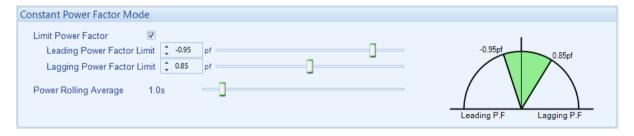
In this mode of exporting power to the Mains (utility); the module varies the amount of reactive power produced by the Generator Bus with regards to maintaining the required power factor. This mode allows the Generator Bus to maintain a constant export power factor if so required. The required power factor is set in SCADA/Generator/Load Levels section, through the Front Panel Running Editor, PLC Functions, or ModBus messages.
