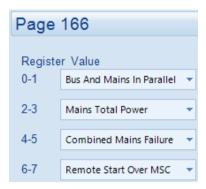
The register address is obtained from the formula: register\_address=page\_number\*256+register\_offset.
