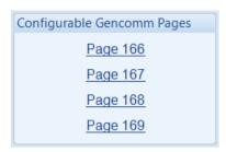
For advanced MODBUS users of the controller, configurable Gencomm pages are available. The intention is to allow the user to create personal collections of data in subsequent registers to minimise the number of MODBUS reads required by the master, and hence speed up data collection.
