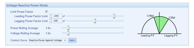
In this mode of exporting power to the Mains (utility); the module varies the amount of reactive power produced by the Generator Bus with regards to the Control Curve depending on the measured voltage.
